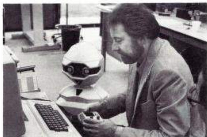
Photo 2. Artist Robert Tinney, at the joystick control, exercises Topo. The Topo form of the Androbot product is an output-only peripheral for Apple-II and Apple-IIIe computers. Topo appears to be examining Robert's actions, a neat trick if Topo could do it. (Topo has no sensors.)
